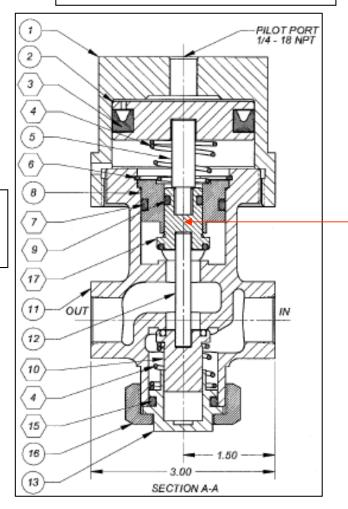
The exhaust port (normally in this location) has been "shaved-off" in this cross-sectional view.
