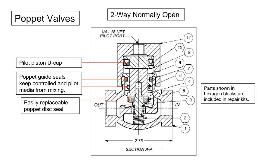
Normally open models feature easy to service design with no need to disturb the plumbing. Simply remove the cap for quick and easy access to all seals.
