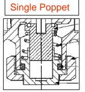
Single poppet design shown at left and above. Larger port size valves utilize a dual poppet design (shown to the right) that helps minimize actuation forces required to open them allowing higher pilot ratios to be achieved.
