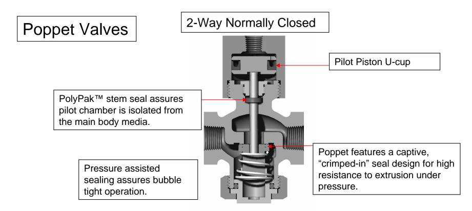
Easy to service design. All models have readily accessible internal parts without the need to disturb the plumbing. Simply remove the bottom hex nut for access to the poppet(s) and spring. Remove the cap for access to the piston and stem seals.
