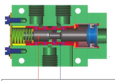
Durable 416 stainless steel spool and patented seal-spacer design assure optimum sealing and long service life.
