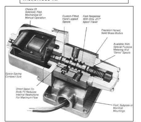
303 stainless steel hand lapped spool has o-ring grooves in the outer lands that are used to keep oil or air inside the body and external contaminants out.
