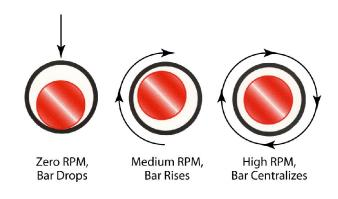
Oil fills the gap between the bar stock and feed tube. As the bar begins to turn, hydrodynamic forces move it toward the center of the feed tube. Centering forces are amplified as bar speed increases. Feed tubes are available in graduated sizes to minimize the bar to feed tube clearance so maximum operating speeds can be achieved.
