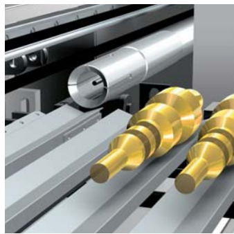
Unloading pusher with clamping sleeve for removing workpieces from the clamping device and positioning them onto the indexed conveyor
