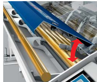
Especially designed loading flap enables reloading of bars without machine stop
